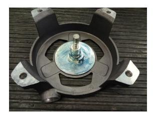
Grease also the upper part of the plastic disk and the central hub of the flash starter,
