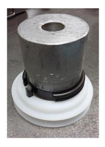
First of all, clean the central thread of the housing with some thinner, to remove any sign of grease from it. Then screw the nut with green glue, grease the bottom of the flash starter and insert the thin plastic disk
