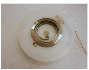
Press in the big spring with the help of a metal cylinder, as in the picture, and a hammer.
