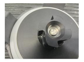
Insert a spacer of di 0,5 mm and put the seeger in its seat. The pulley driver should have some play, if the flash starter has too much play add a spacer of the right thickness.
