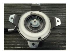
Pre-charge the spring making only one turn of the rope and let it exit from its seat with the help of a hook
