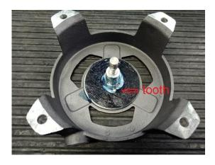
Insert the pulley paying attention to fix the small spring in the tooth of picture 2 of previous page
